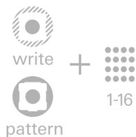
hold write + pattern and press 1-16 to paste the active pattern to the corresponding new slot.
